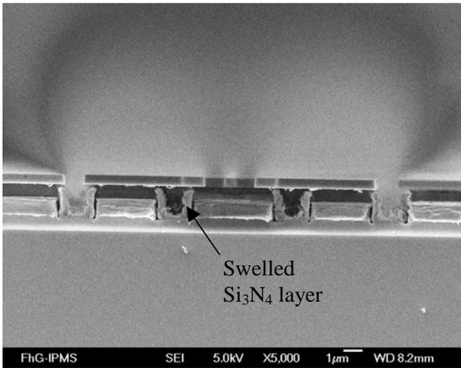
**Figure 2: The result of vapor HF etching of a device with an etch stop layer of Si<sub>3</sub>N<sub>4</sub>, showing incompatibility with the release process**
