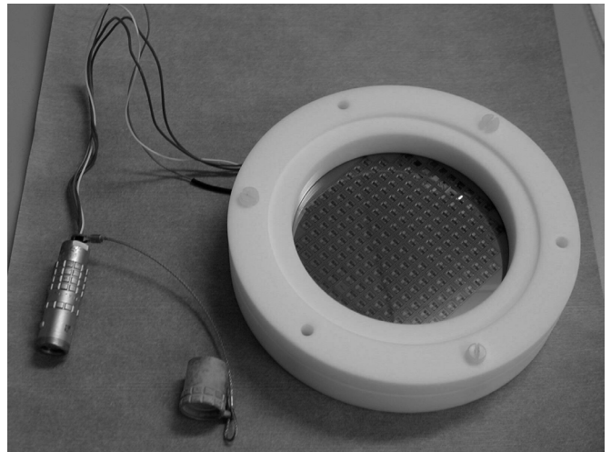
Fig. 1: Our Teflon chuck with a clamped wafer and the cables for the heating foil and the temperature sensor.
