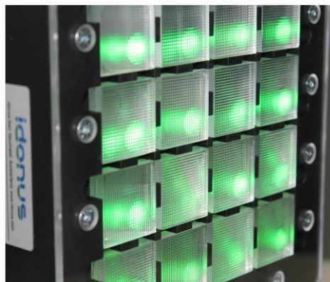
Customized LED-based illumination • Our client uses this matrix of green (550 nm) and IR (850 nm) LEDs for non-telecentric illumination of wide display panels (400 × 400 mm 2 ).
